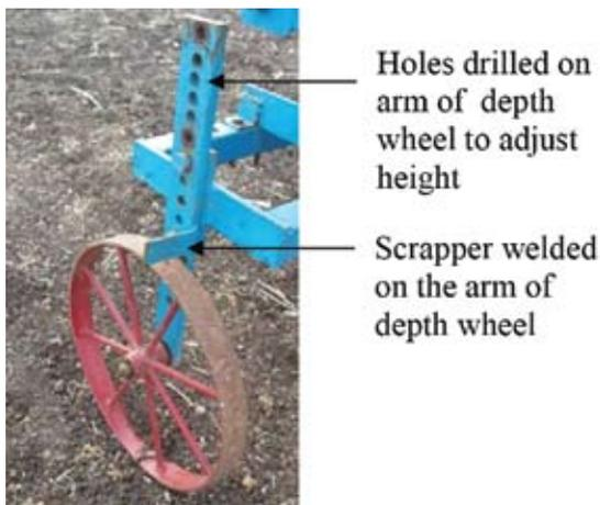
Fig. 2 : Holes drilled and scrapper welded on the brace/arm of ground wheel
