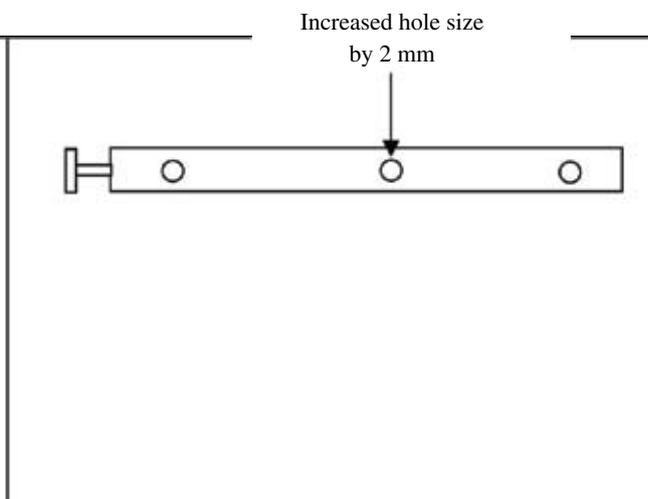
Fig. 5 : Fertilizer control lever
