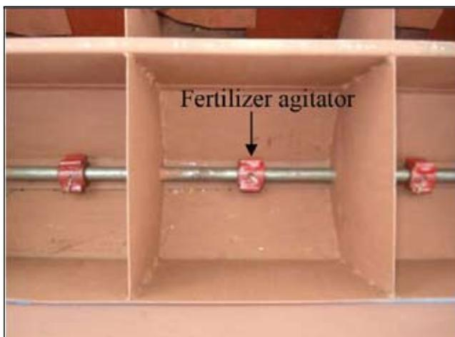
Fig. 4 : Refined fertilizer agitator fitted on fertilizer shaft
