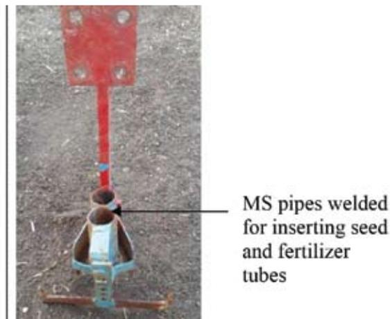
Fig. 3 : Boot with seed and fertilizer delivery pipes
